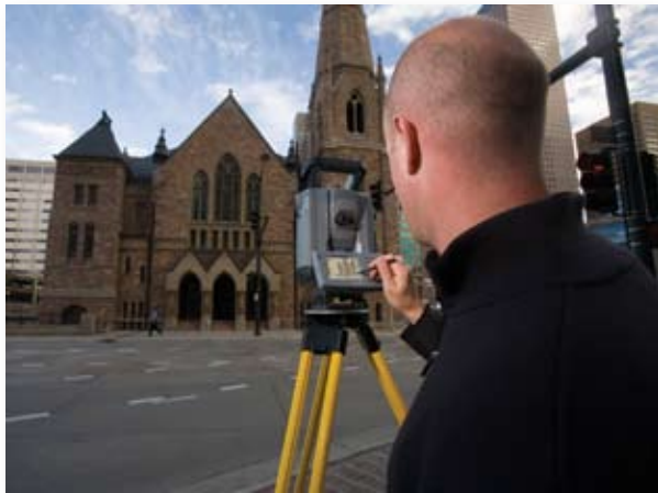
Surveying a church using Trimble total station
