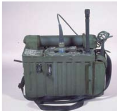
Figure 2. Manpack Global GPS exhibited at National Museum of American History, Division of Medicine and Science [http://americanhistory.si.edu/collections/object.sfm?key=35&objkey=220].
